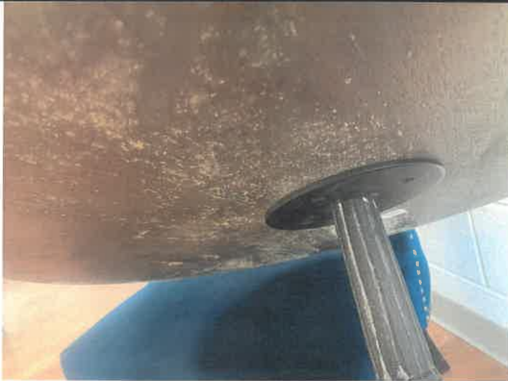
Photo 13: Visible mold on the bottom side of the table in the lounge area
